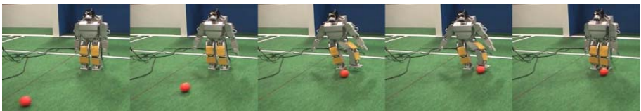
Fig. 4. An experimental result of a trapping skill
