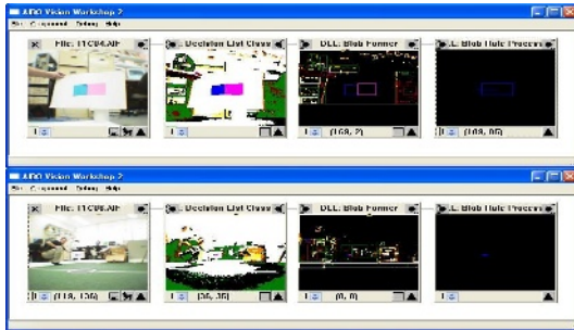
Fig. 6. AIBO Vision Workshop 2 running sideways beacon detection code. The XOD to find sideways beacons (flags) differs only in one word to the XOD used to locate normal beacons
