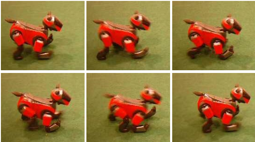
Fig. 3. The Aibo ERS-210 walking with 311 mm/s
