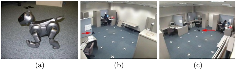
Fig. 1. The Sony ERS-210A entertainment robot (a) and views from two of the Smart House overhead cameras (b),(c). Note the large overlapping region and the white crosses marked on the carpet. Arrows indicate the position of the robot
