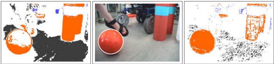
Fig. 4. Left: Colour segmentation of a ball, a bare foot and red posts. Middle: Circle detected in the left image. Right: Colour segmentation after training
