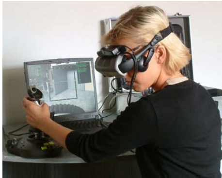
Fig. 6. Orpheus Operator's Station for Telepresence Control
